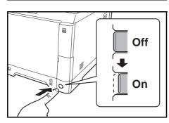
**6** Turn the main power switch on. The machine begins to warm up.
